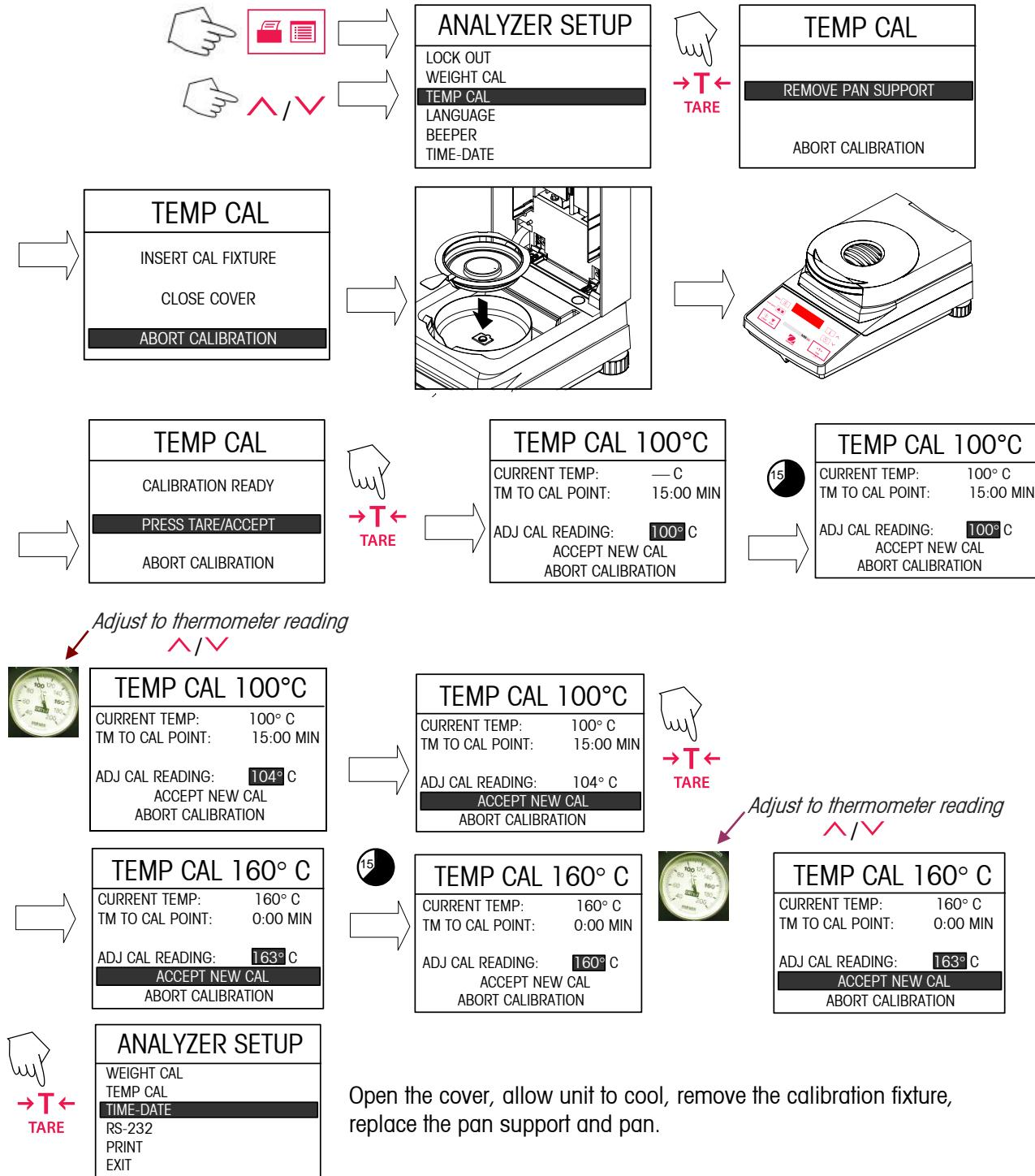
Open the cover, allow unit to cool, remove the calibration fixture, replace the pan support and pan.
