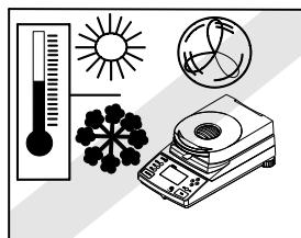
**DO NOT** install the Moisture Analyzer next to:
