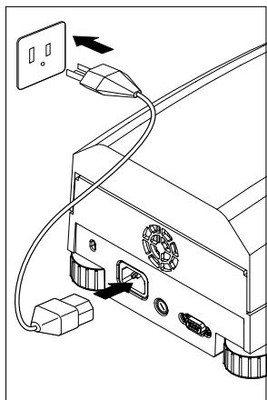
Connect power cord as shown. The MB35 is operational when power is applied. The display remains off until the On/Off button is pressed.
