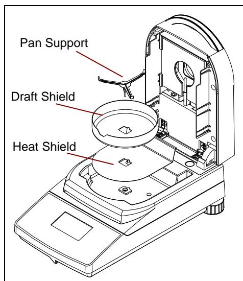
Install the heat shield, draft shield and pan support as shown. Turn the pan support until it engages in the locked position.
