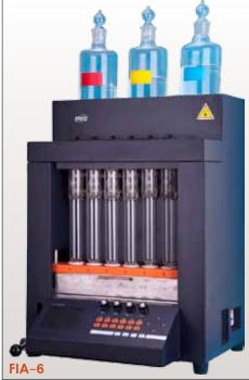
FIA-6 Fiber Analyzer is an analysis Instrument used to the crude fiber content of samples through acidic or alkaline hydrolysis, flushing and filter process. FIA-6 functions include automatic solution adding, automatic pre-heating and so on. Infrared tube heating is used, and high-precision soak extraction and filter ensure test precision; high-definition color LCD screen displays temperature and time.
