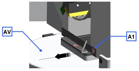
Fig. 16: Removing the discharge flange
