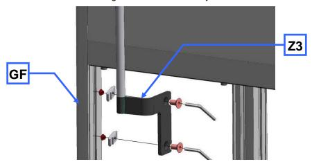
Fig. 21: Fastening the cyclone support
