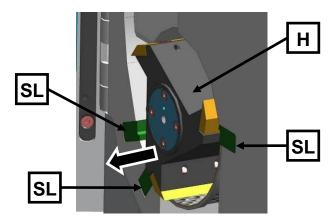
Fig. 7: Freely rotate the rotor
