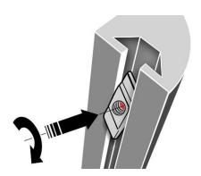
Fig. 20: Turning the sliding block
