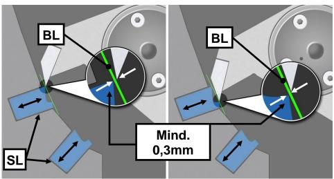
Fig. 8: Adjusting the cutting gaps
