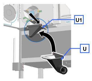
Fig. 17: Fastening the discharge flange
