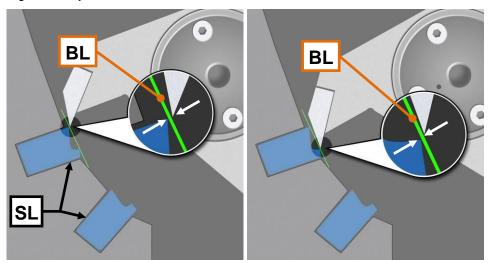
Fig. 3: Checking the cutting gap
