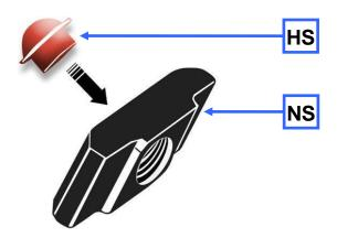
Fig. 18: Inserting the plug for the sliding block
