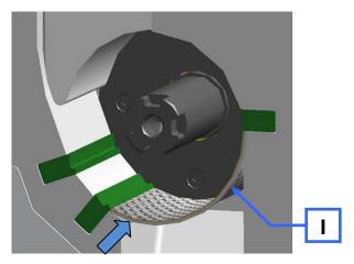
Fig. 12: Inserting the bottom sieve
