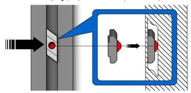
Fig. 19: Inserting the sliding block
