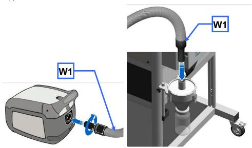
Fig. 24: Connecting the industrial vacuum cleaner
