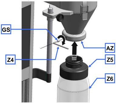
Fig. 25: Inserting the wide mouth bottle adapter
