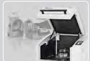
RETSCH Vibratory Disc Mills for medium-hard, brittle and hard-tough materials with feed sizes up to 15 mm achieve grind sizes down to 0.04 mm. This makes them ideally suited for sample preparation to spectral analyses. RETSCH Disc Mills achieve grind sizes of approx. 0.1 mm.
