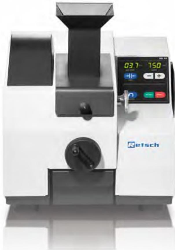
The BB 50 is designed for a very efficient and convenient size reduction process. The **variable speed** can be set between **550 and 950 min<sup>-1</sup>** to adapt the crushing process to sample requirements. The possibility to **reverse the rotating direction** is helpful if too much sample material has been fed to the crusher causing it to block. The simple push of a button restarts the process. There is no need to empty the crushing chamber manually.
