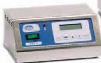
Complete unit with: Dry-block connected to a programmable process unit, (time and temperature) rack support for tubes and fume extractor.
