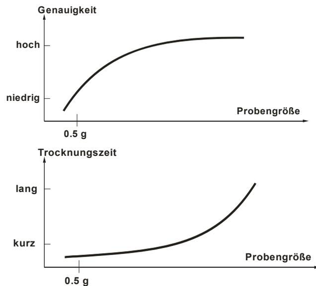
The heavier the originally weighted-in quantity, the more accurate the result (example of an ideal sample):
