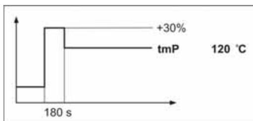
Drying temperature **tmP** adjustable from 40°C-160°C.
