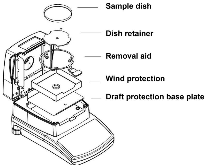
Put on the dish retainer carefully, ensuring correct positioning:
