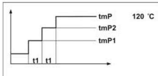
Adjustable parameters include the drying temperature **tmP**, warming-up steps **tmP1** and **tmP2** as well as the heating-up time **t1** and **t2** between the single steps.
